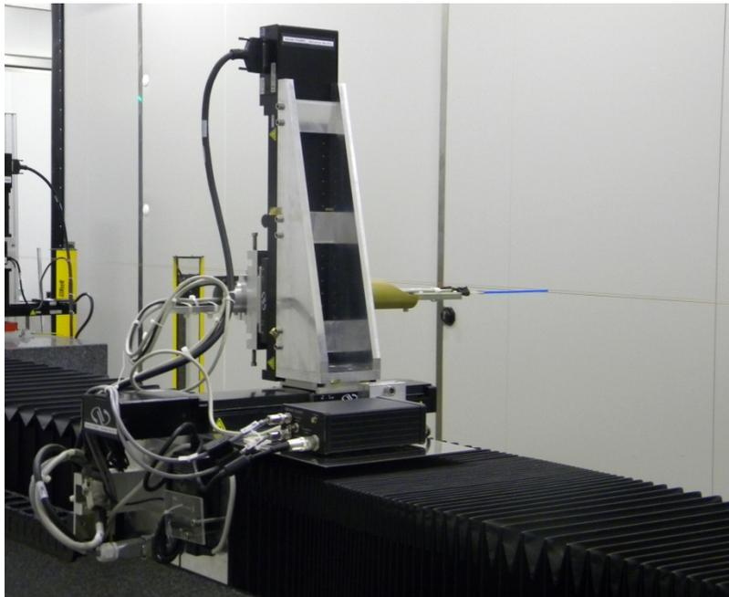
Figure : Senis A.G. Ultra Low Transducer mounted on the measurement bench.
