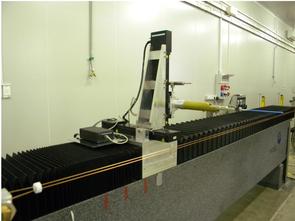
Figure : The Hall Probe and Flip-Coil large benches.
